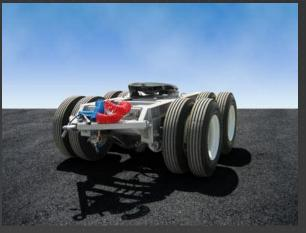
25 X 25 thousand pounds with pneumatic suspension Dolly made with high strength carbon steel.
