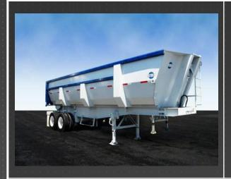
Sturdy trailer for heavier tasks of the construction industry and mining, made in 2 versions, 24 and 30 meters. Cu
